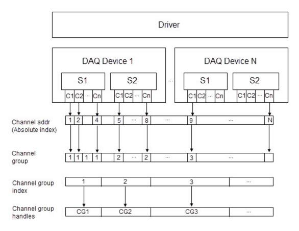
channel group could include all channels of all subsystems in a single device, or all channels of the same type of subsystem across several devices.
